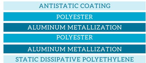
The heavy metallization structure is essentially that of a shielding bag but with opaque, thick layers of metallization. Nylon is regularly used in place of Tyvek or polyester, providing the needed strength at a lower cost than Tyvek.
